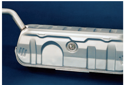
Fig. 12: Motor vehicle fuel tank made of steel sheet with Aluminium-Silicon coating (AS)
