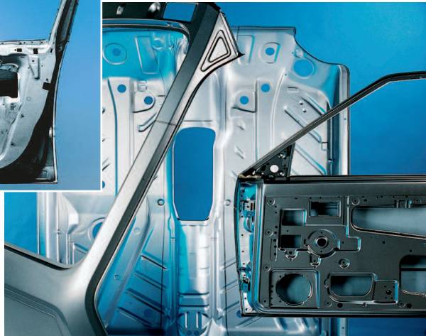
Fig. 14: Chassis parts, in part laser-welded, made of hot-dip galvanized sheets
