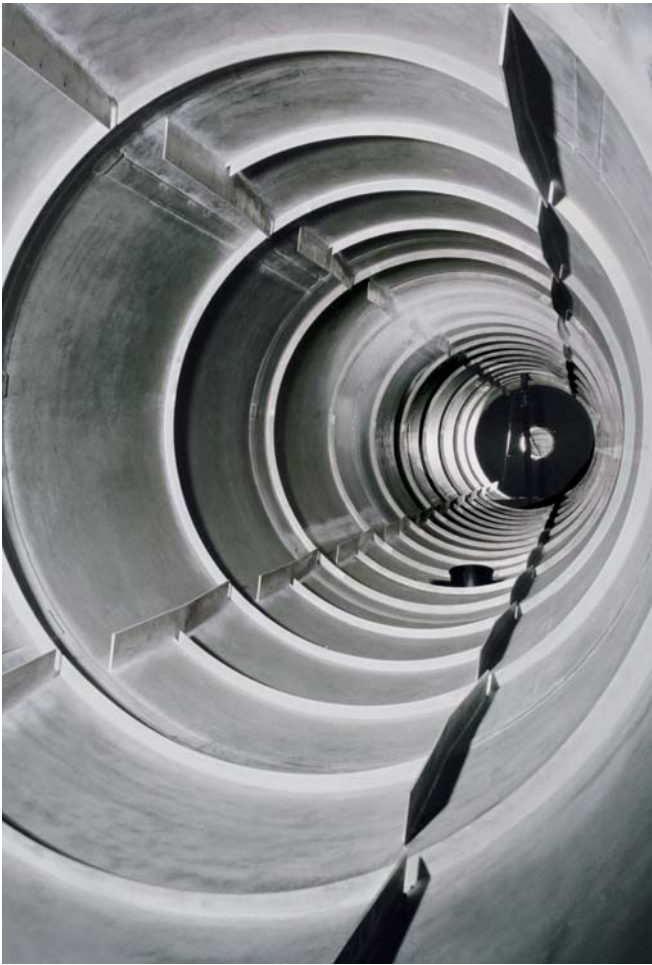
Figure 2: Examples of the uses of clad plate Top: Inside view of a shell ring for a chemical reactor, clad with zirconium 702 low oxygen by explosion bonding Right: Inside view of a flue-gas scrubber, clad with NiCr23Mo16Al by hot-roll bonding
