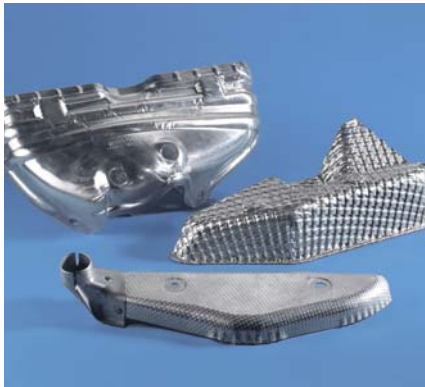
Automotive heat shield made of aluminium-clad steel sheet (DC01) Properties: corrosion-resistant, high reflection of thermal radiation
