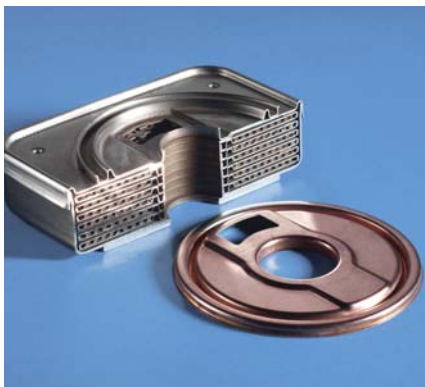
Automotive oil cooler made of copper-clad corrosion-resistant steel (X5CrNi18-10) Properties: copper functions as brazing filler material
