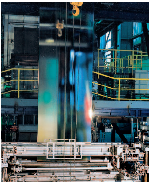
Strip after leaving the coating pot and passing the gas-knives
