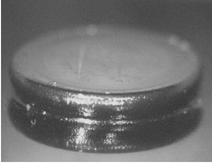
Fig. 9: Clinch connection without damaging the coating
