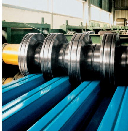
Fig. 8: Roll forming of organic coil coated steel sheet
